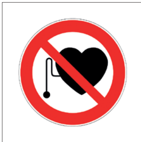
"Forbidden for people with cardiac pace- maker" acc. to BGV A8 P11
