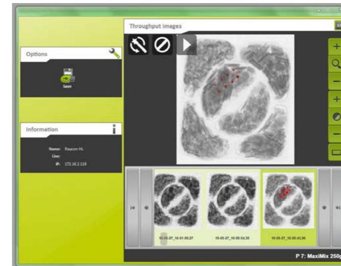
Download from the stored x-ray images of good and rejected products on RAYCON inspection system.
