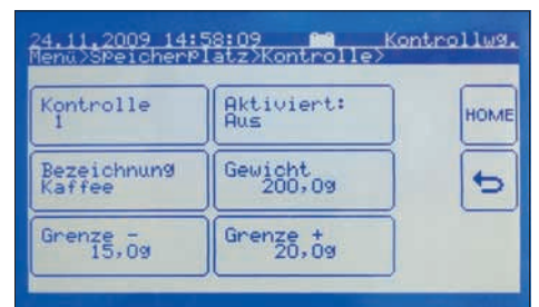
40 memories for each mode, for checkweighing, pre-tare, reference weight, target weight when dispensing, etc.
